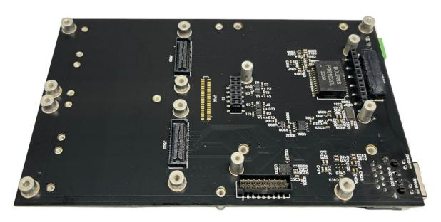
The Base Board is a carrier board for the <u>AMD</u> Kria<sup>™</sup> K26 SOM Module. Most SOM IO Pins are spent for the 4x PMOD (HDIO) and the 2x ZMOD (HPIO) connectors.
