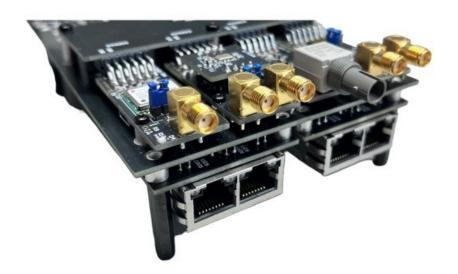
The two main interfaces modules which AIONYX is using, are compatible with two already defined interfaces on the development board market. One is the <u>Digilent</u> Pmod™ Interface and the other on the <u>Digilent</u> Zmod™ Interface compatible with the connector of the SYZYGY specification. So the Pm and Zm modules can also be used with other base or development boards on the market.
